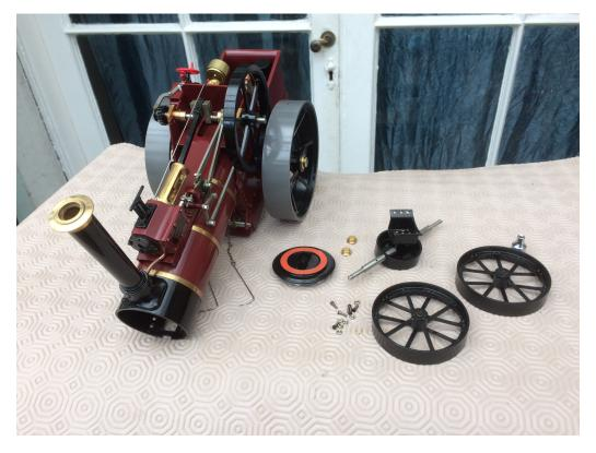
Maxitrak Ltd 10-11 Larkstore Park, Lodge Road, Staplehurst, Kent, TN12 0QY Tel: 01580 893030 Email info@maxitrak.com Check the fit of the wheels inside the front rolls, they should just slide in. Remove paint from the wheels if necessary.
