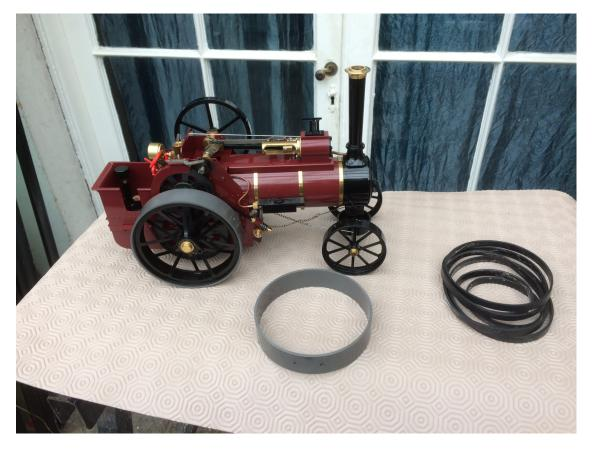
Remove the steering chains from the front axle.
