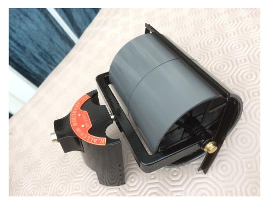
There are five bolts to go into the perch bracket on each side, the two nearest the boiler are 2 mm dia and fitted with M2 nuts and bolts. The third (center) bolt must be drilled 1.6 mm dia and tapped out to M2, there is no room for a nut on the inside of this bolt as it would foul the smokebox door. The fourth and fifth bolts are dummy and are bolted into
